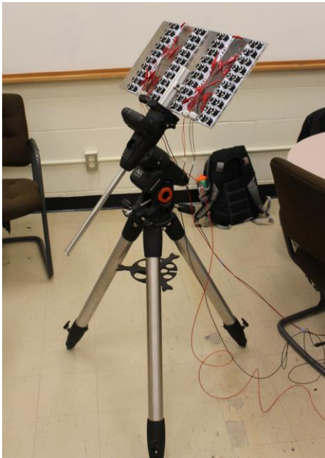
Figure 2. A photograph of the Beaver Signal, the prototype beacon. The LED array is mounted on top of the Celestron AVX motorized telescope mount, with the power supply out of the picture to the right. The array measures 58.4 cm by 30.5 cm, and the entire assembly stands 1.4 meters tall.
