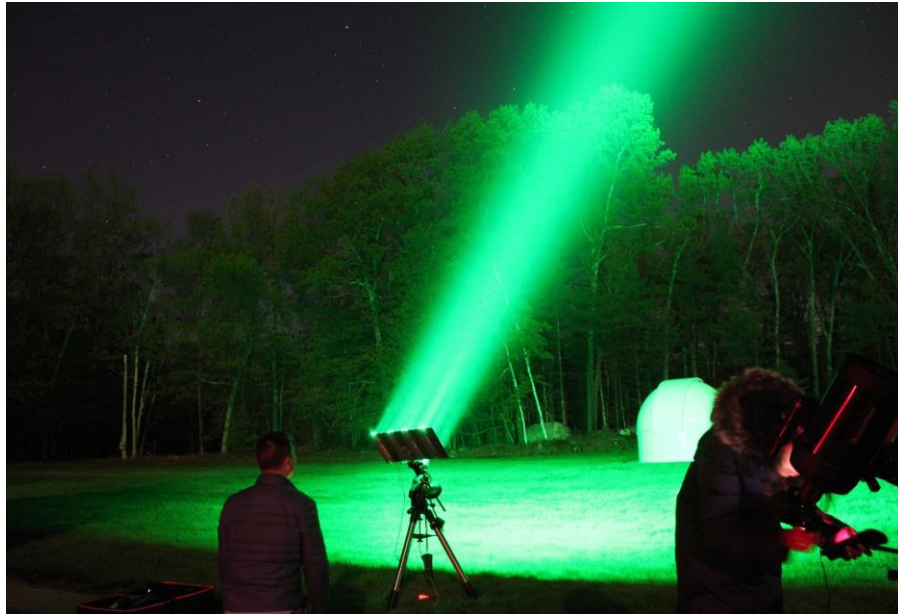
Figure 5. The beacon during testing at Wallace Astrophysical Observatory. The LED array is mounted on the AVX in the center of the frame. The power supply and computer controller are out of the frame to the bottom.
