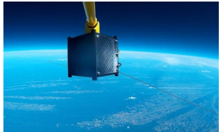
Figure 7. This image of the CubeSat prototype was captured at an altitude of 16 km. We note that the apparent curvature of the horizon is caused by the wide-angle lens of the camera.
