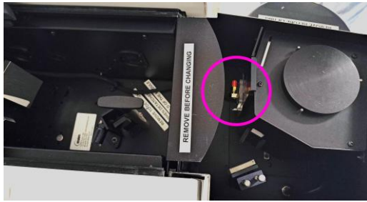
Figure 5. Transmissivity test setup. The antenna is highlighted with the pink circle.
