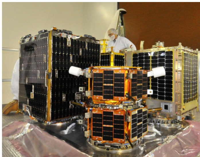
Figure 1. FASTRAC (Center) mated onto the adapter plate of STP-S26 (Hernandez, 2011).
