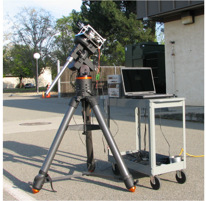
Figure 2. Photograph of pseudo-STARE prototype payload shown in 1 attached to Celestron telescope mount. Adjacent to the payload is an Orion finder-scope used for fine pointing. The cart next to the mount holds two power supplies to deliver the 3.3, 5.0, and 12.0 Volt lines that the Colony II provides in addition to the computer that serves as the data acquisition system.
