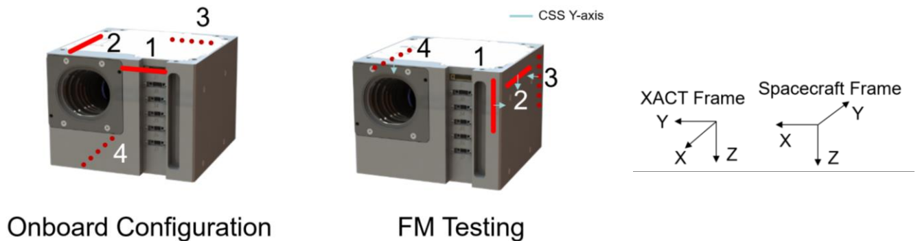
Figure 9. Rotated sun sensor positions to enable FM ground testing.
